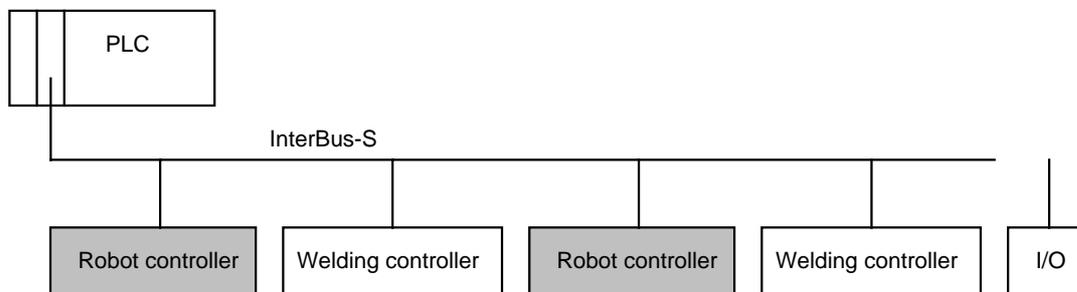
**Figure 3: Description of a typical system configuration**
